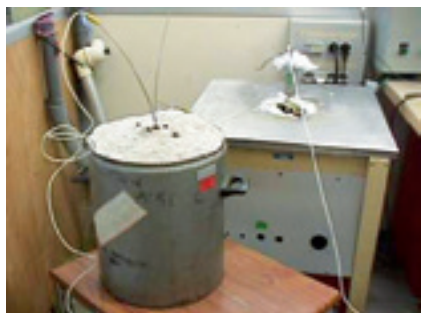
Calibration by comparison: salted bath
